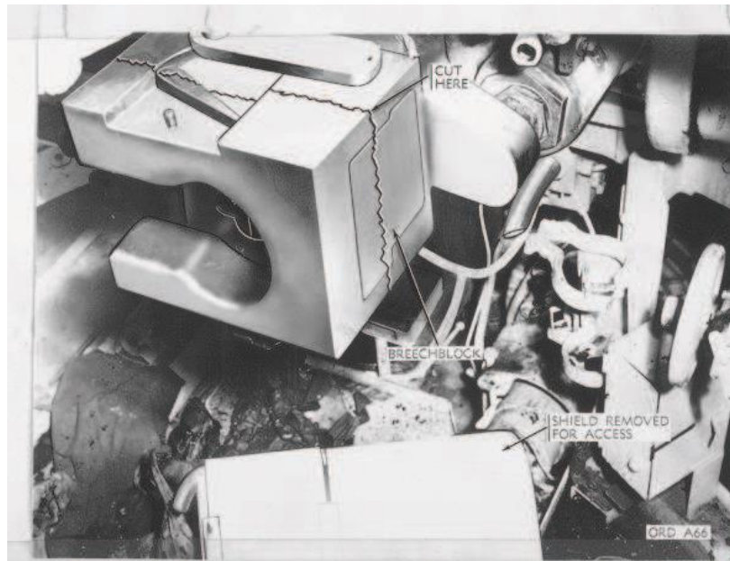
Figure 8. Interrupted Thread Breechblock
